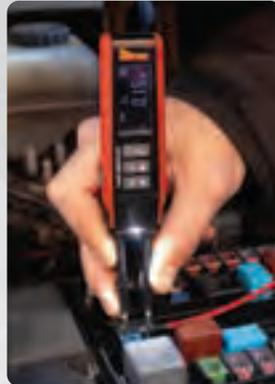
**LA PARTIE SUPÉRIEURE DE L'OUTIL INDIQUE INACTIF, ACTIF OU OUVERT POUR UN DIAGNOSTIC RAPIDE DU FUSIBLE.**
